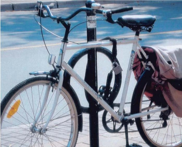
*Bicycle racks should be constructed of a good quality single locking post-and-ring design (source: Pat Bailey and Sharon Latham).*
