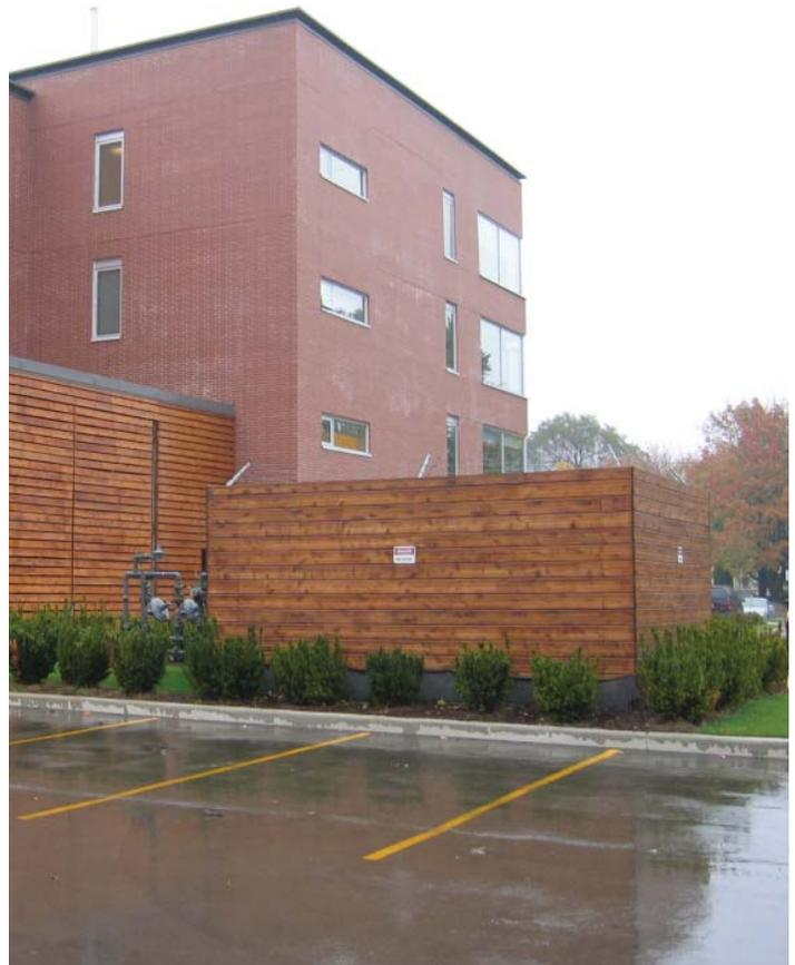
Service and loading areas should be screened by appropriately designed walls or enclosures and should be integrated into building designs.
