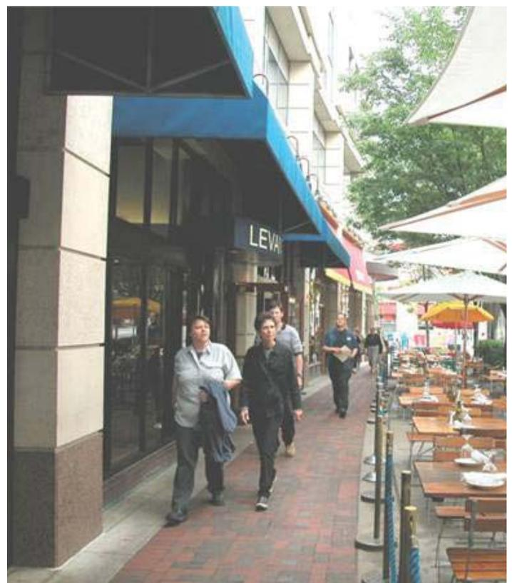
*Canopies are recommended to provide weather protection to pedestrians and to help articulate building elevations and principal building entrances.*
