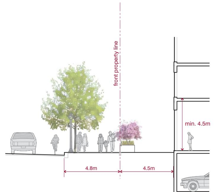
Where the ground floor of a residential unit is level with the sidewalk, 4.5 metres is recommended for the setback and the ground floor height.
