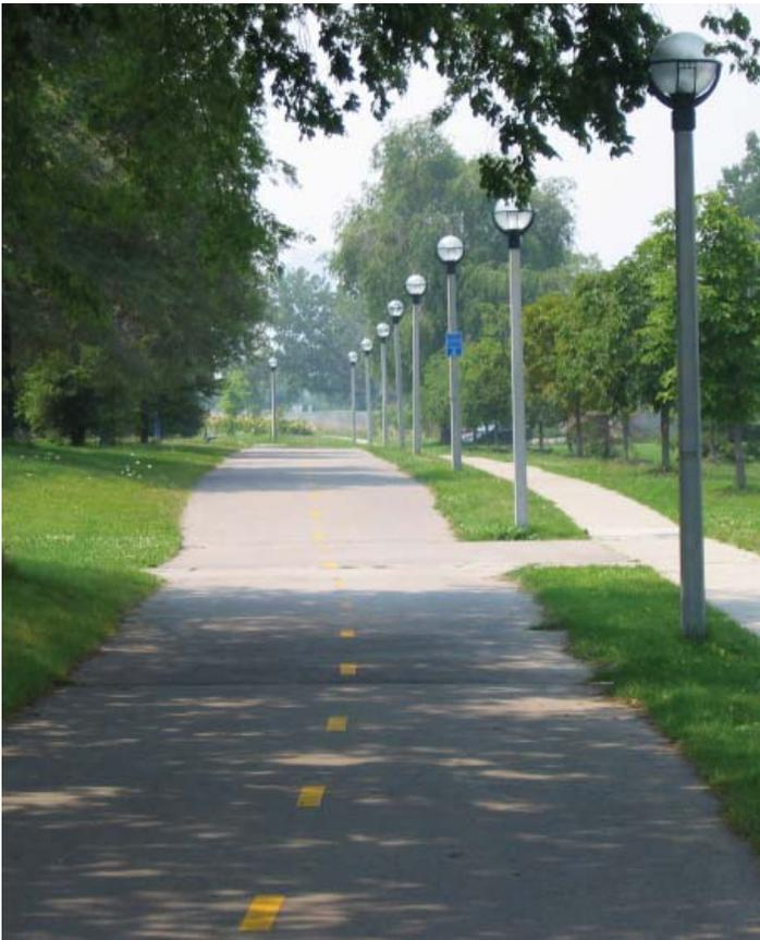
Two-way trails designed for use by cyclists should be a minimum of 3.0 metres wide.
